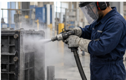
Dry ice blasting
